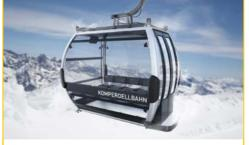
Numbers / Dates / Facts: Bottom station: 1,442 m Mid station: 1,610 m Top station: 1,982 m Length of 1st section: 566 m Length of 2nd section: 2,075 m Total length: 2,641 m Altitude difference: 540 m Transport capacity: 3,000 persons/hour (3,500 persons/h in the final stage) Number of supports: 20 supports Travel time: 10.5 minutes Construction costs: 50 million euros
